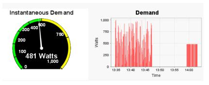
This part shows the Instantaneous Demand attribute as received from Mock Meter ETRX3USB as a meter dial as well as plotted in a chart against time. This visualization is updated periodically at an interval of 5 seconds.
