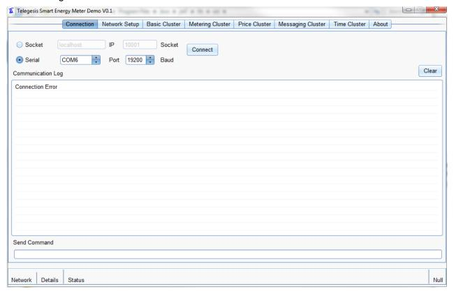
Click on the "Serial" radio button and select the serial port from the adjacent field. Click "Connect" to attempt to connect.
