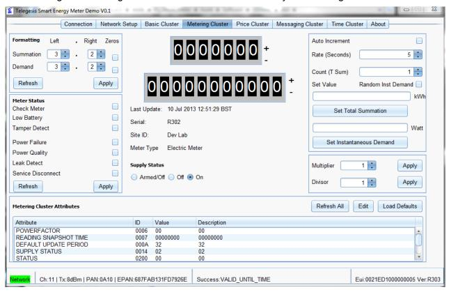
To set the meter to auto-increment its current summation attribute the "Auto Increment" check box can be checked which will make the application update the Current Summation attribute as specified in the field "Count (T Sum)" and at the rate specified by "Rate (Seconds)" field. If the "Random Inst Demand" button is checked a random value between 0 and 1000 watts will be set in the Instantaneous Demand attribute at each interval as specified by the "Rate (Seconds)" field.
