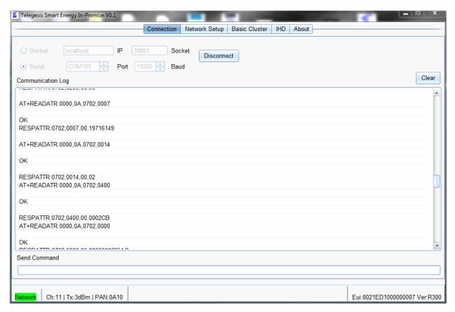
If the selected Serial Port does not connect to an IPD ETRX3USB then an error is shown in the status bar.
