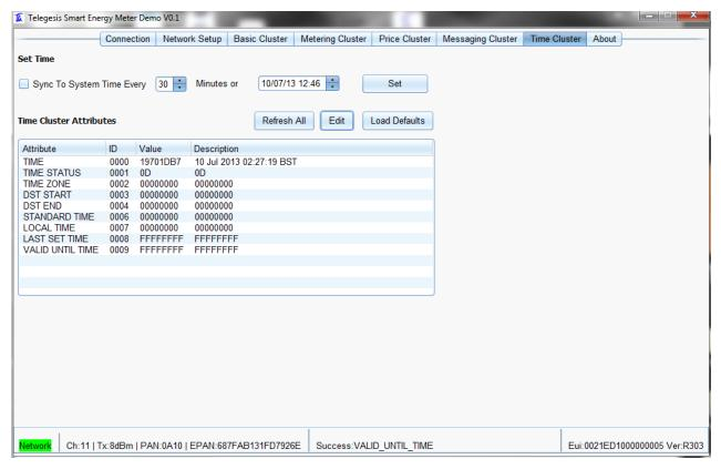
Check the checkbox "Sync Time to System Time" to enable syncing the time of the Mock Meter with the computer. The time in the Mock Meter may drift over time so the application allows for syncing the time with the PC periodically.
