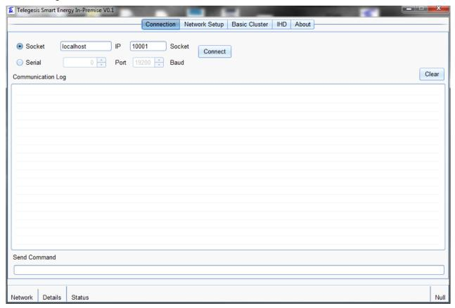
Click on the "Serial" radio button and select the serial port from the adjacent field. Click "Connect" to attempt to connect.
