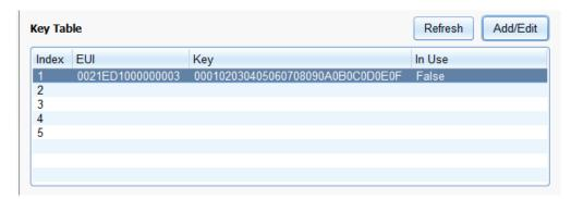
The field "In Use" changes to "True" once the device has joined and has successfully completed the CBKE process.
