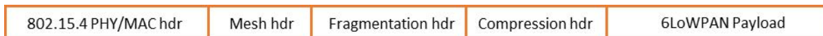
Figure 3.5. 6LoWPAN Packet Containing Mesh Header, a Fragmentation Header, and a Compression Header
