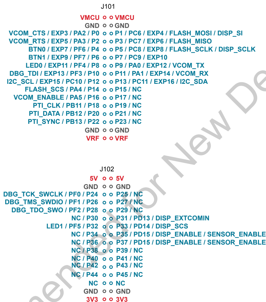
Figure 3.2. Breakout Pad Pin Mapping
