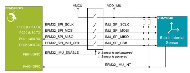
Figure 3.8. ICM-20648 Six-axis Inertial Sensor
