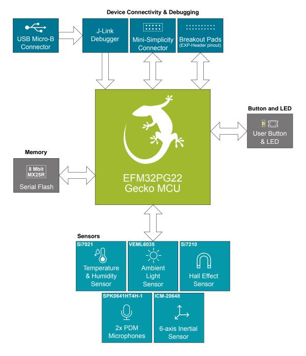
Figure 3.1. Kit Block Diagram
