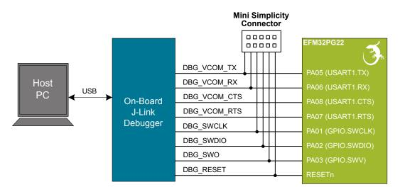
Figure 3.12. On-Board Debugger Connections
