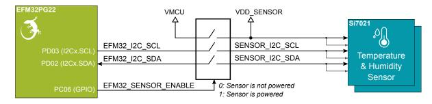
Figure 3.4. Si7021 Relative Humidity and Temperature Sensor
