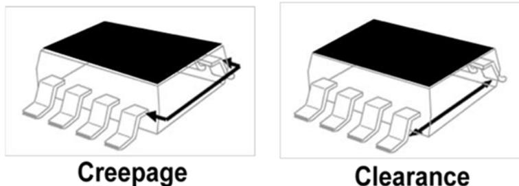
**FIGURE 1: Creepage and Clearance Distances**
