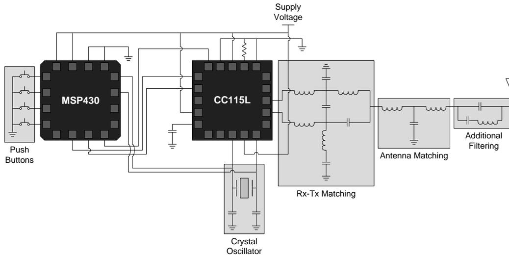
**Figure 3. Partial Discrete Transmit Solution (TI CC115L + MSP430)**
