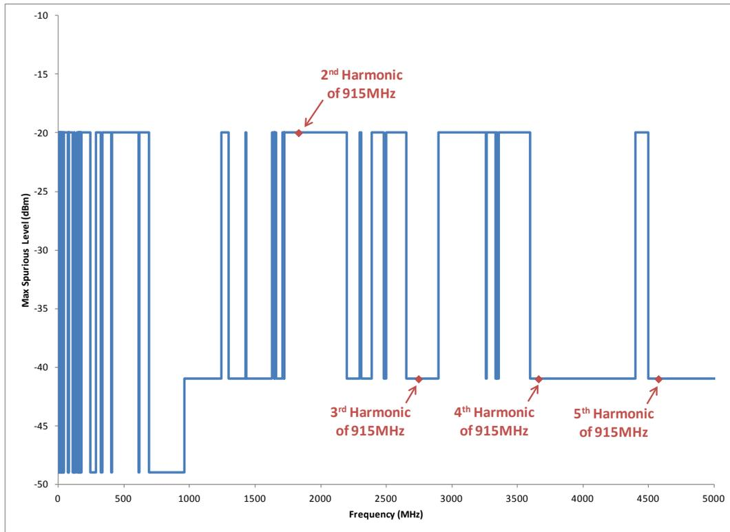
**Figure 2. FCC Spurious Level Restrictions by Frequency**
