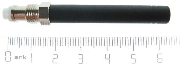
Figure 1: As radio frequencies are reduced, antenna sizes increase proportionally
