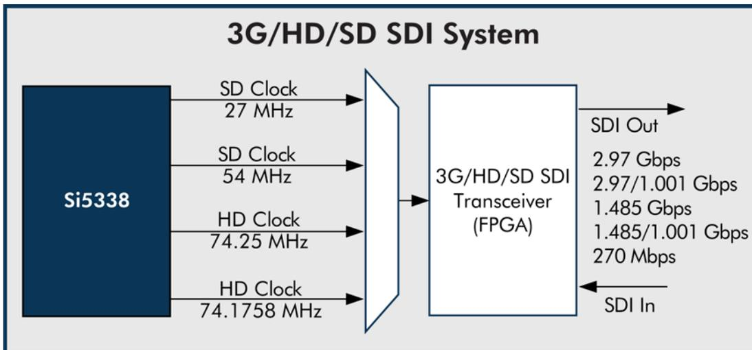
**Figure 7.** Si5338 Simplifies Broadcast Video Timing Architecture
