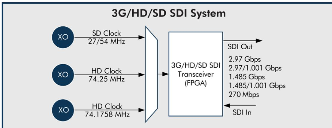
**Figure 2.** Traditional Timing Architecture in Broadcast Video Applications
