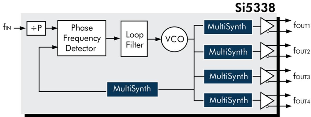
**Figure 4.** Si5338 Any-Rate, Any-Output Clock Generator Architecture
