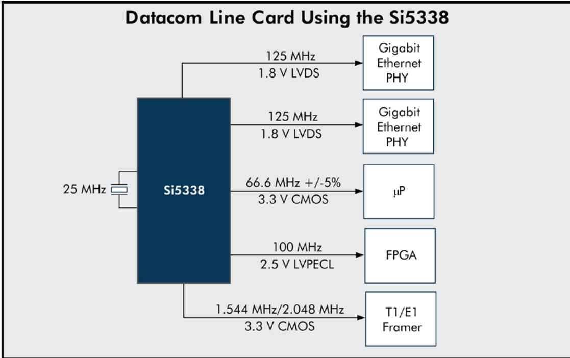
**Figure 6.** Si5338 Simplifies Communication and Networking Timing Architecture
