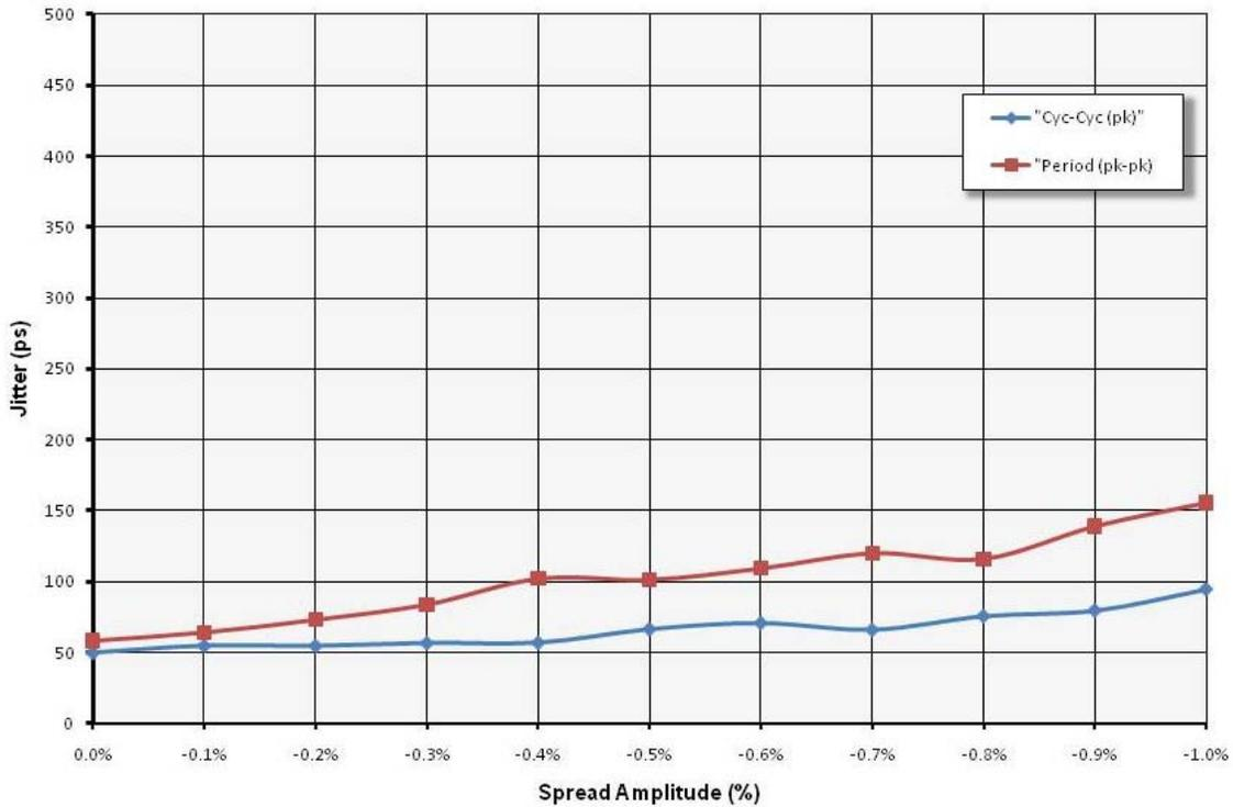
**Figure 3. SSCG Minimizes Period and Cycle-to-Cycle Jitter**
