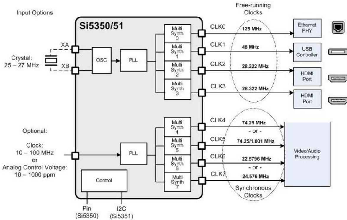
**Figure 4. Si5350/51 Programmable General Purpose Clock IC**
