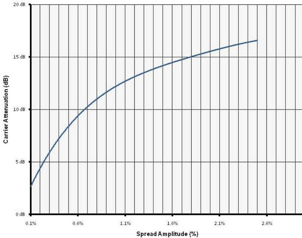
**Figure 2. SSCG Reduces EMI at any Single Frequency**
