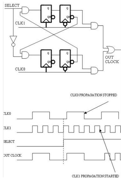
**Figure 2. Traditional Glitch-Free Shifting Circuit**
