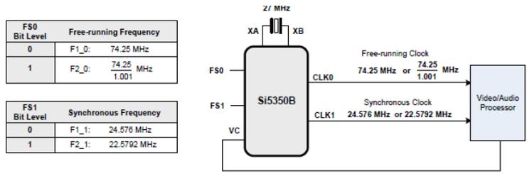
**Figure 4. Si5350/51 Simultaneously Generates Audio and Video Clocks**
