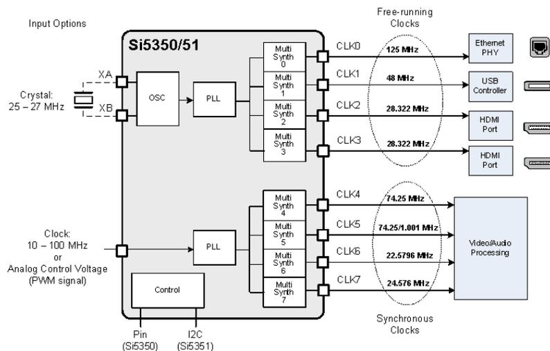
Figure 3. Si5350/51 Generates Timing for Multiple Clock Domains
