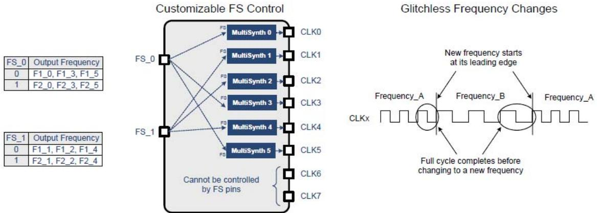
**Figure 5. Custom Control Pins and Glitchless Frequency Change**
