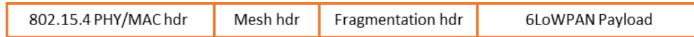
Figure 6. 6LoWPAN Packet Representing Subsequent Fragments that Do Not Contain Any Information about the IPv6 Header
