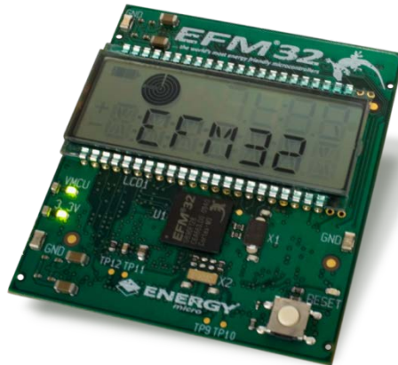
Figure 7: EFM32 directly driving a 160 segment LCD display
