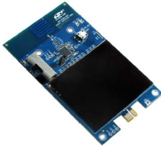
Figure 3. Example of Energy Harvesting Reference Design
