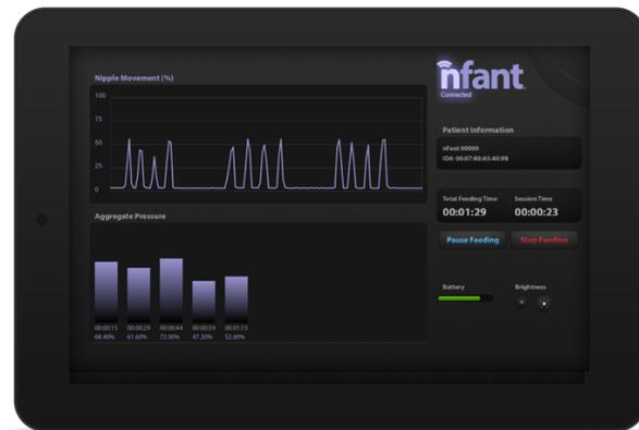
*Via a Bluetooth Smart wireless transmitter installed in an electronic nipple on a baby bottle, information on the state of an infant born prematurely can be sent to a nearby monitor for use by an attending nurse or saved for later evaluation by a physician.*
