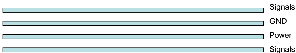
Figure 15: Typical 4-layer PCB construction
