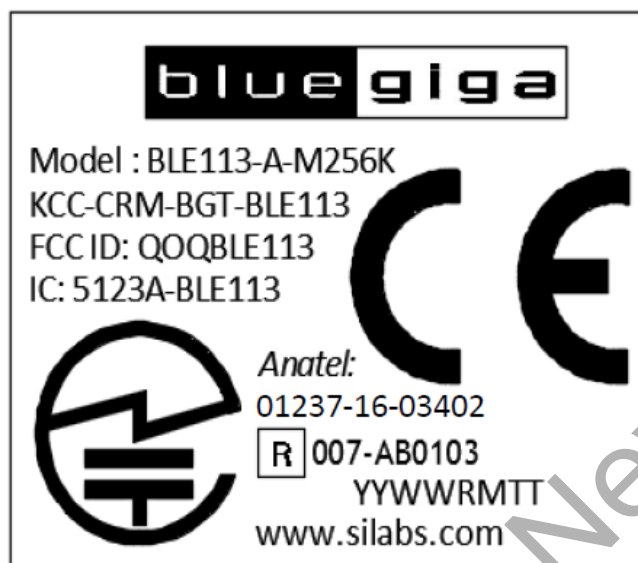
Figure 22: BLE113 package marking
